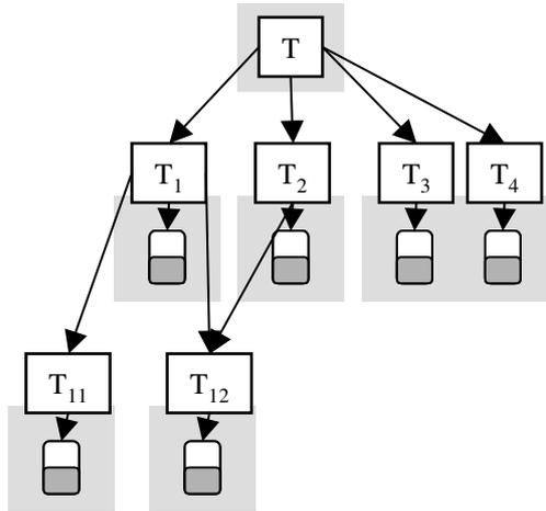
**Fig. 2** Nested transaction. The Root node T spawns four children. T<sub>1</sub> spawns two more children resulting in four leaf nodes. It can be seen that T<sub>12</sub> actually works as sub-transaction for both T<sub>1</sub> and T<sub>2</sub>. T<sub>3</sub> and T<sub>4</sub> work at the same node
