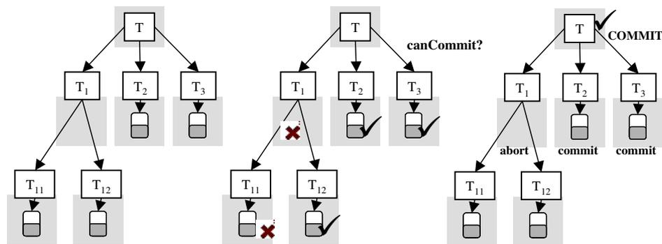
**Fig. 4.** Two-Phase Commit protocol in a Nested Transaction. Since  $T_{11}$  and  $T_{12}$  do not receive a final commit or abort, they abort by default after a timeout
