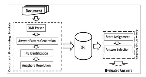
Figure 2. Question Answering based Machine Reading System Architecture
