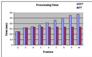
Figure 3. The processing time for BPF algorithm vs IPF Algorithm.
